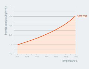
\*Thermal conductivity measured with laser flash ; results would be significantly lower with hot plate.
