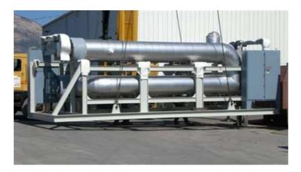
Steam superheating is probably one of the most common applications for electric process circulation heaters because they keep the steam dry and at 100% quality – making it perfect for direct use in your processes.
