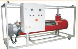
GCP pass superheaters consist of a GCB heating group assembled on a steel or stainless steel tubular body, of suitable flange, bed and entry, exit and purge tubulatures, threaded or flanged. The fluid to be heater circulates inside the same, guided by the deflectors at intervals in the
